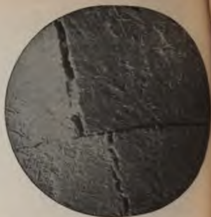
FIG. 4.—BRITTLE PLATE BROKEN AT RIGHT ANGLES, THE ROUGH CLEAVAGES OF CRYSTALS. Natural size.
